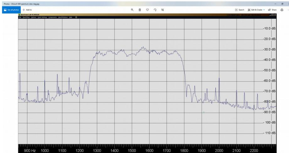
A popular mode for EMCOMM traffic on 80m is **MFSK-32**, operating at 32 baud, 120 wpm, and a bandwidth of 630 Hz. If permitted, the speed **MFSK-128** (125 baud, 480 wpm, 1920 Hz bandwidth) would yield very fast data traffic, but taking up almost 2 kHz of spectrum is not advised
